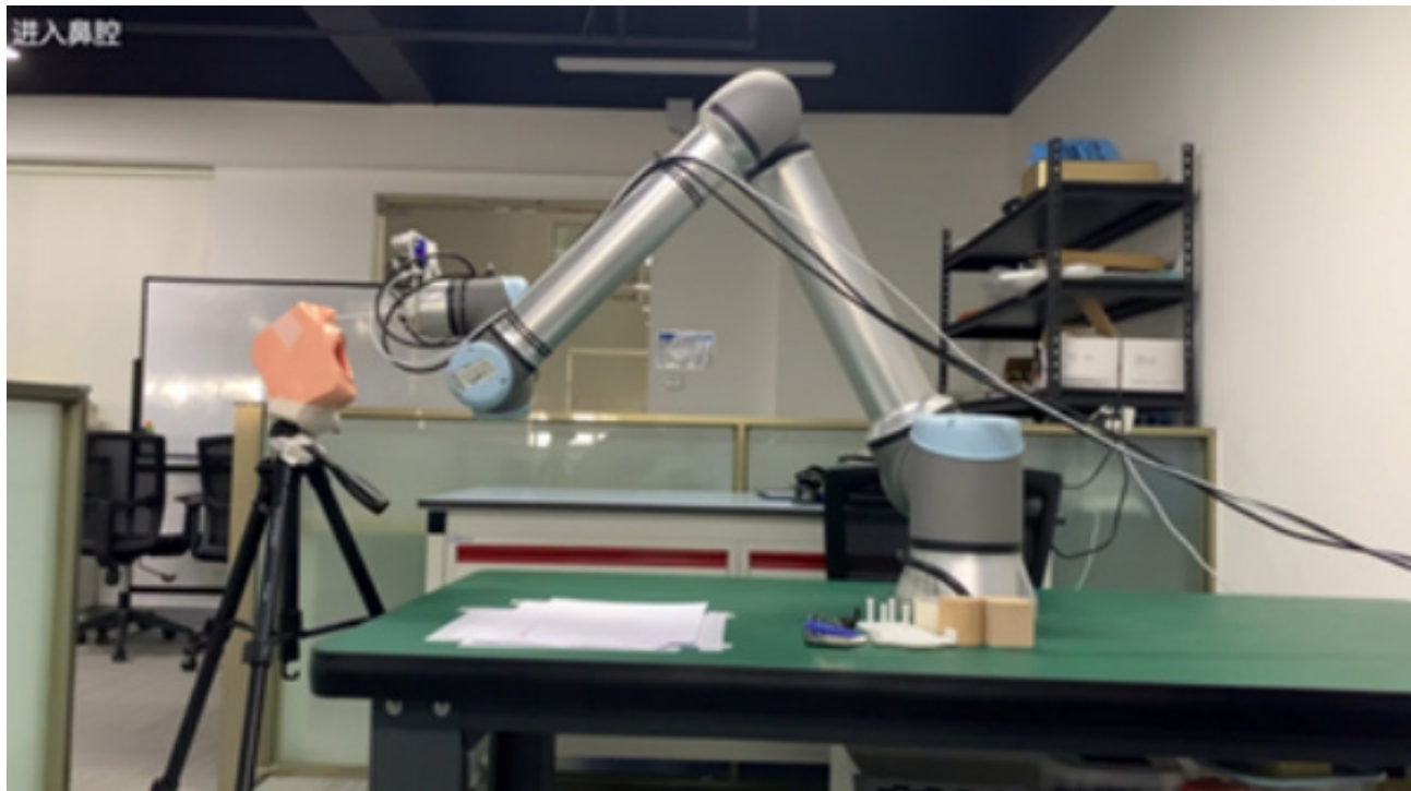
Figure 8 Experiment of the Robotic Arm Entering the Nasal Cavity
