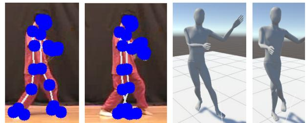
**Fig. 8. MediaPipe misidentified the coordinates of both legs in subsequent frames, causing a deviation in the performance effect in Unity3D**
