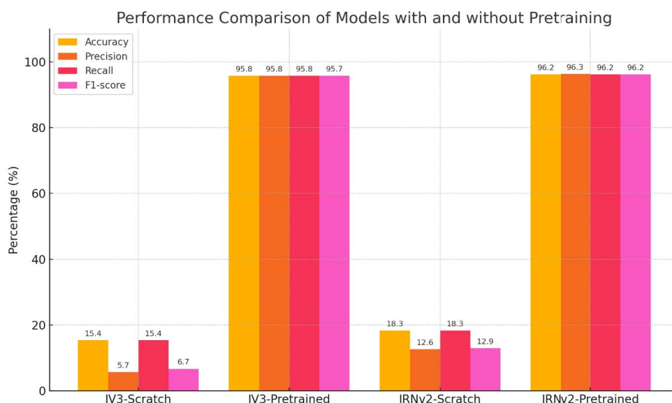
Fig. 2 Performance comparison of InceptionV3 and InceptionResNetV2 with and without pretraining (Picture credit : Original)
