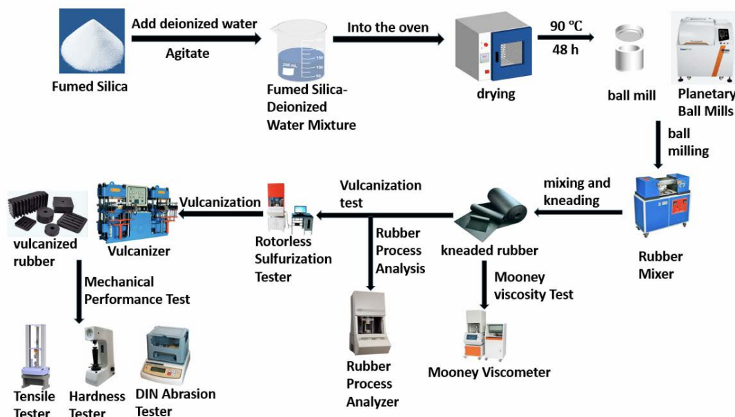
Fig. 1 Schematic workflow for fumed-silica hydration, mixing and testing[3]
