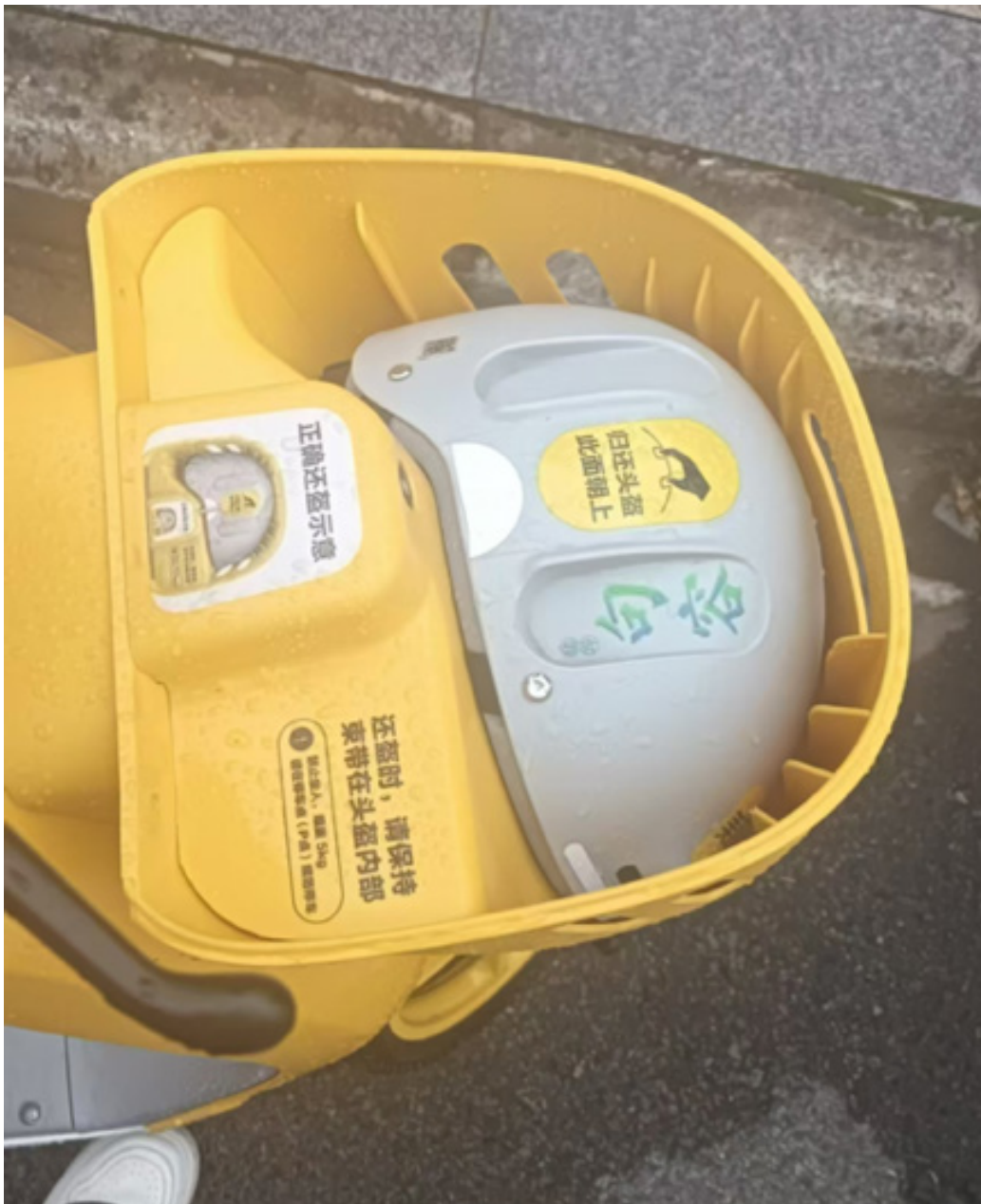
Figure 9. Illustration of the arrangement of the basket and helmet on the upgraded shared electric scooter.
